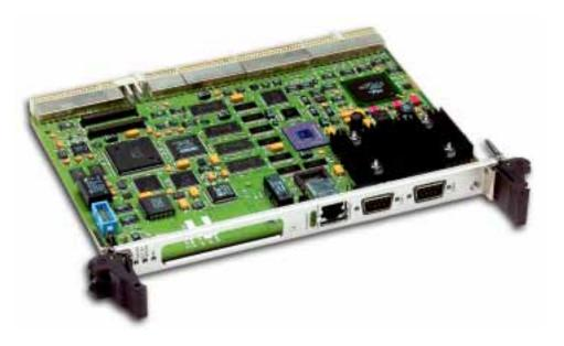
**Denali** <sup>TM</sup> is a 6U cPCI board with PowerPC 603e @ 200MHz processor (optional PowerPC 740 @ 266MHz). The board has 64 Mbyte of SDRAM, 8 Mbyte of flash memory, 512Kbyte socketed flash, 10BaseT/ 100BaseTX ETHERNET with interface on an RJ-45 connector, 32K byte NVRAM/RTC, two RS-232C ports with interface to DB-9 connectors, PMC interface, ATM SAR with dual J5 interfaces, PCI bridge to cPCI bus, watch dog timer, and interface to 8 digital I/O signals.
