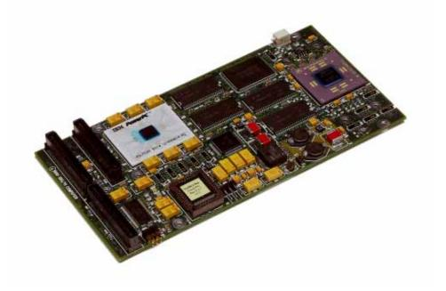
**Palomar II**  $^{\text{TM}}$  packs the performance of the PowerPC 750 processor and 64MB of SDRAM into a PMC compliant form-factor (149mm x 74mm). The Palomar II design includes 1MB L2 Cache to boost application performance.
