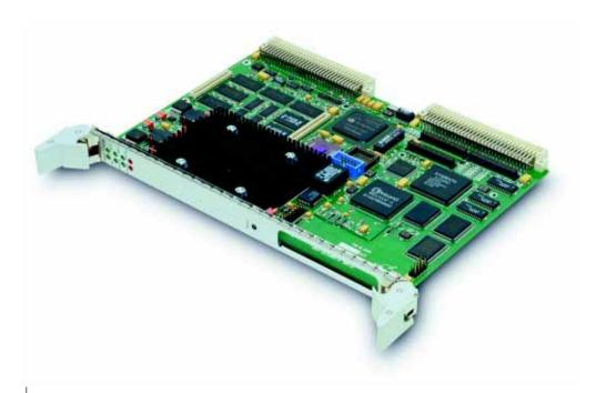
**Power-4C** TM is a high performance VMEbus single board computer with the PowerPC 604R processor, a 512KB L2 cache, and synchronous DRAM to provide unparalleled performance in a single board computer.
