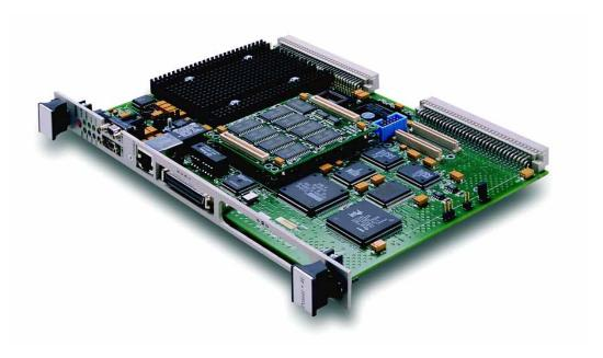
**Power-4e** TM is a high performance VMEbus single board computer with front panel I/O. The Power-4e couples a 300MHz processor with a 512KB L2 cache and EDO DRAM to provide cost-effective performance in a single board computer.
